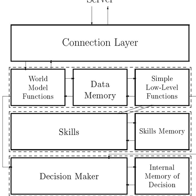
**Fig. 1.** The agent four layered architecture. From top : (1) Connection layer (2) World model layer (3) Skills layer (4) Decision making layer
